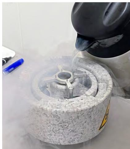
\* The inside of the ethane cup is also filled with liquid nitrogen (evaporates in a short time).
