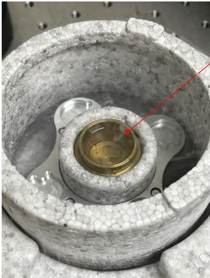
Make sure the ethane cup is filled with liquid ethane
