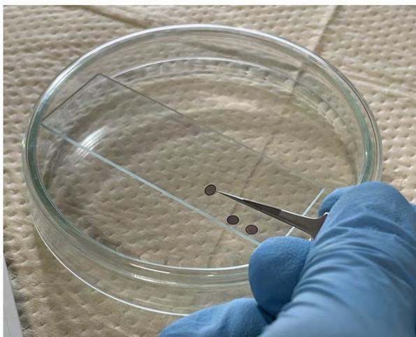
When pinching the grid with tweezers, pinch the outer periphery to avoid scratches. Pay close attention to the grid, as it is easy to bend (**bent grids cannot be used for measurements**).
