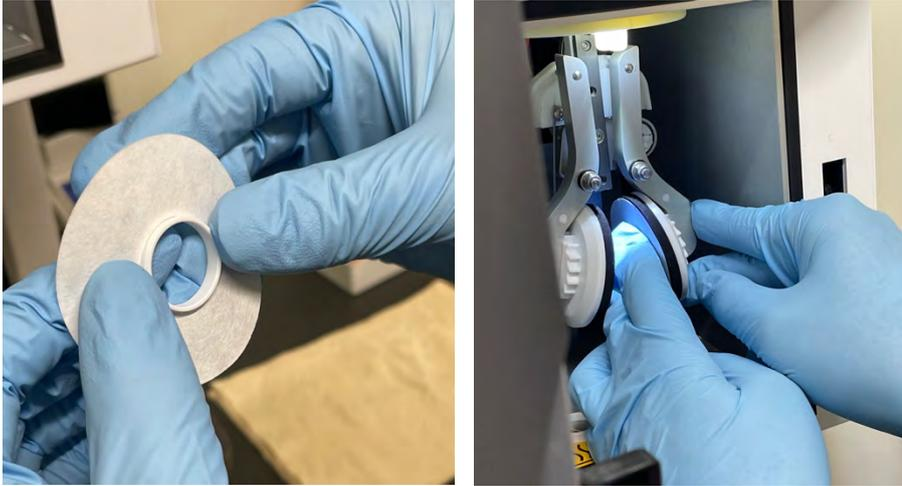
\* It is safer to align the front and back of the filter paper in a certain direction each time.
